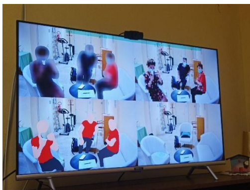
Figure 2. Session with users showing in real time the privacy preservation algorithms: blurring, pixelation, avatar, and invisibility.
